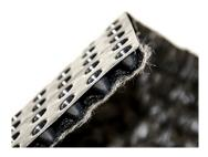
ARDEX DRS 10 GC is a cuspated HDPE sheet with a geotextile layer that provides effective drainage and protection against backfill. ARDEX DRS 10 GC provides high compressive strength to resist heavy pressure loads. The geotextile layer of ARDEX DRS 10 GC effectively protects against backfill materials while allowing water to migrate into the core channel providing consistent ventilation and hydrostatic relief.
